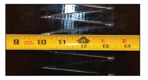
**STEP 1:** Prepare the press by placing a piece of silicone paper on the platen. Align the belt cover side <u>facing up</u> so that there is a  $\frac{1}{4}$ " to  $\frac{1}{2}$ " space between the tip of the finger and the joint.
